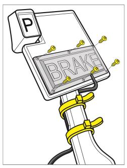
Secure the brake pad wire to the bottom side of the assembly using cable ties. Slowly lower the pedal into PARK and recheck the lead. Readjust the cable ties if necessary.
