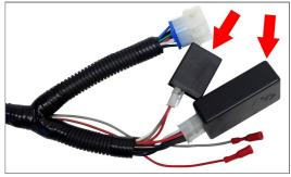
3. Remove the jumper harness from the 9-pin turn signal connector on the RHOX plug and play harness.
